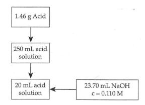
$n(NaOH) = 0.110 \times 0.02370$ = 2.607 × 10<sup>-3</sup> mol Ratio of acid to NaOH = 2 : 1  $n(Acid) = \frac{1}{2} \times n(NaOH)$ = 1.3035 × 10<sup>-3</sup> mol in 20 mL In 250 mL  $n(Acid) = 1.3035 \times 10^{-3} \times \frac{250}{20}$ = 0.01629 mol  $M_r = \frac{m}{n} = \frac{1.46}{0.01629} = 89.6 \text{ g mol}^{-1}$
